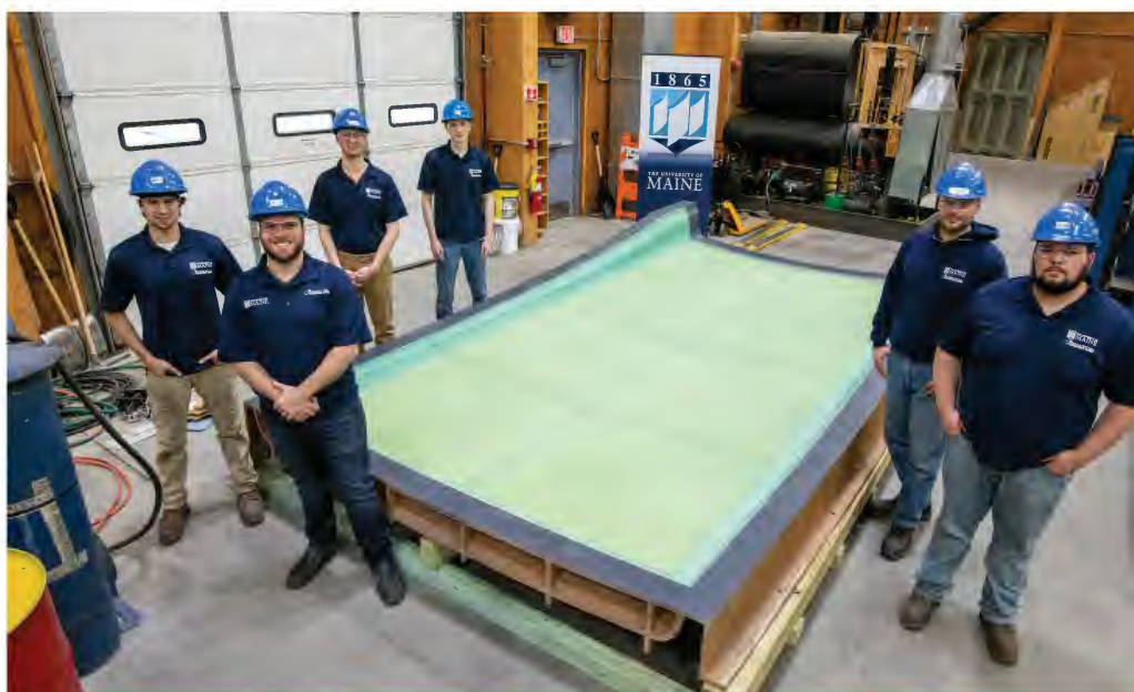
Advanced Structures and Composites Center students and staff show off a boat roof from a 3D-printed mold made with a new biomaterial, nanocellulose reinforced polylactic acid, developed at UMaine.
