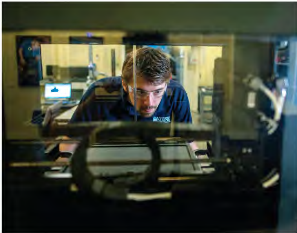
At the Center for Additive Manufacturing of Metals, three machines use metal powder mixed with wax and a polymer binder to create structures with similar properties to metal parts produced by casting or subtractive processes, such as milling or turning.
